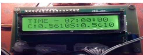
Fig4: Power consumes & power saves displayed in LCD unit.
