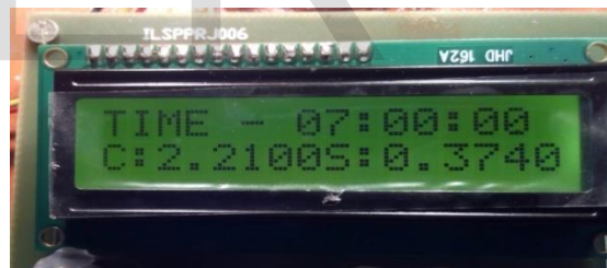
Fig8: Power consumes & power saves displayed in LCD unit.
